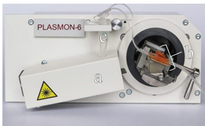
Figure 2: SPR spectrometer "Plasmon-6", which includes an optical unit containing laser and photodiode (a), measuring flow cell in the Kretschmann configuration (b) and a holder for the test sample (c)
